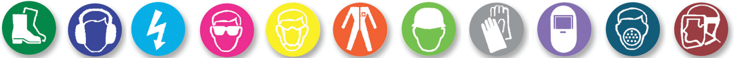
Protective Footwear Ear Protectors Use RCD Eye Protection Dust Mask Overalls Safety Helmet Gloves Welding Mask Respirator Face Shield
